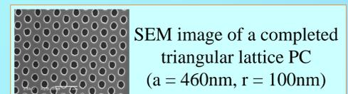
SEM image of a completed triangular lattice PC
