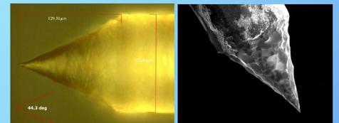
Optical (left) and SEM (right) images of a completed silica tip with opening angle of 44.3° approximately
