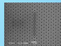
SEM image of CL-7 inside a triangular 2D PC (a = 460nm, r = 100nm)
