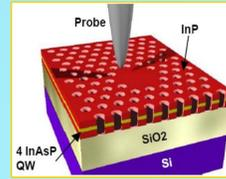
Optical characterization at a sub-wavelength scale
