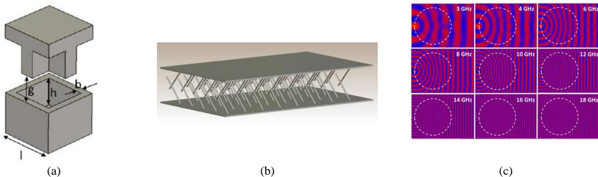
Fig. 1 – (a) Unit cell of a glide-symmetric structure. (b) Example of anisotropic glide-symmetric metasurface. (c) UWB glide-symmetric Luneburg lens transforming a cylindrical wave into a plane wave for directive radiation at its end (the phase of the fields is shown in the picture).
