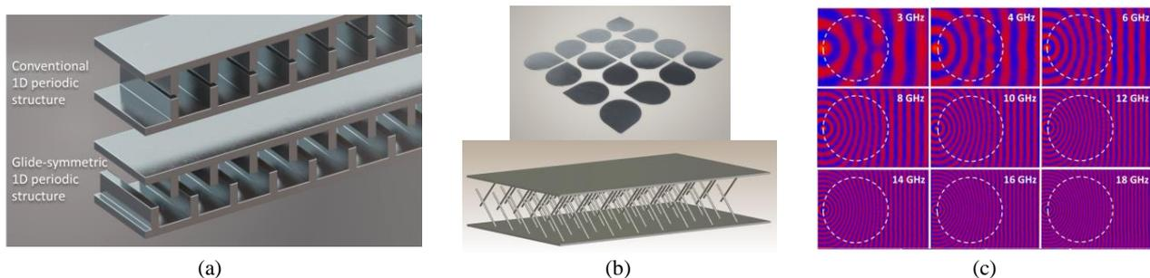
Fig. 1 – (a) Conventional periodic structure and glide-symmetric structure. (b) Examples of screw-symmetric and anisotropic glide-symmetric metasurface. (c) UWB glide-symmetric Luneburg lens transforming a cylindrical wave into a plane wave for directive radiation at its end (the phase of the fields is shown in the picture).
