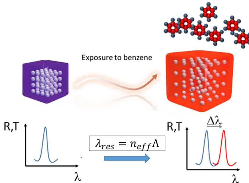
Fig 1. Sketch of the sensing principle: a polymer-based photonic crystal – PhC – (periodic arrangement of dielectric materials) swells upon exposure to VOC (Benzene for example), leading to a change of its geometric parameters. The monitoring of the resonance wavelength shift allows following the PhC deformation and determining the VOC concentration.
