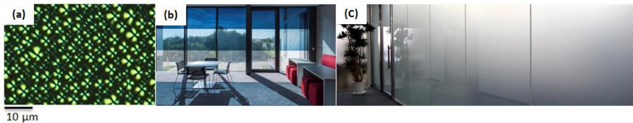
Figure 1: (a) Polarizing optical micrograph of toric focal conic domains in liquid crystal films. (b) Image of an insulating window. (c) Image of controllable scattering in a window for privacy applications.
