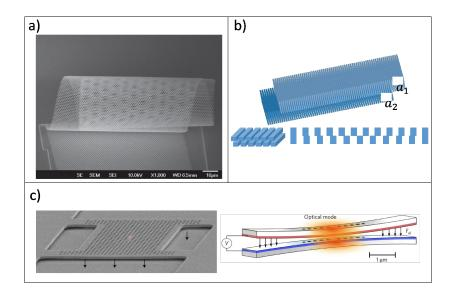
**Different technological routes to fabricate "Photonic Moiré**": a) 2D "tilted" moiré obtained by self-winding of a CP membrane at INL [3], b) schematic views of a 1D moiré obtained by double nanostructuring with alignment c) NOEMS (Nano Opto-Electro-Mechanical Systems) technologies can also be used to couple CPs [4]
