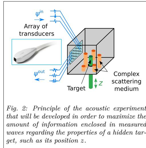
*Fig. 2: Principle of the acoustic experiment that will be developed in order to maximize the amount of information enclosed in measured waves regarding the properties of a hidden target, such as its position  $z$ .*
